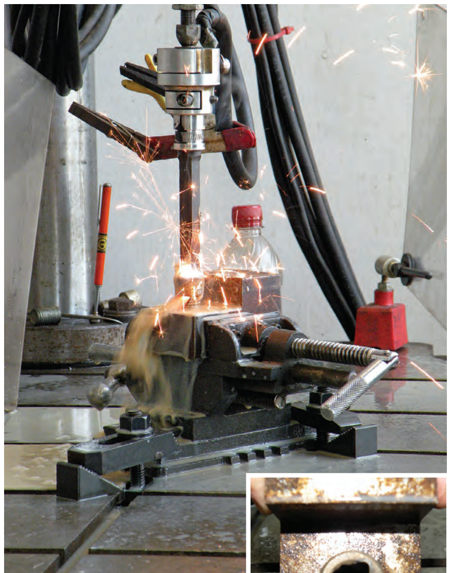
Above, Ken Guthrie, owner of CBG Maintenance Services LLC in Norfolk, stands back while the company's Cammann metal disintegration machine goes to work. In the other photos the machine is cleaning out a hydraulic pan, shown at right.
